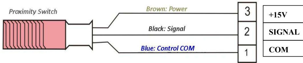
Fig 3-2 NPN proximity switch connection
